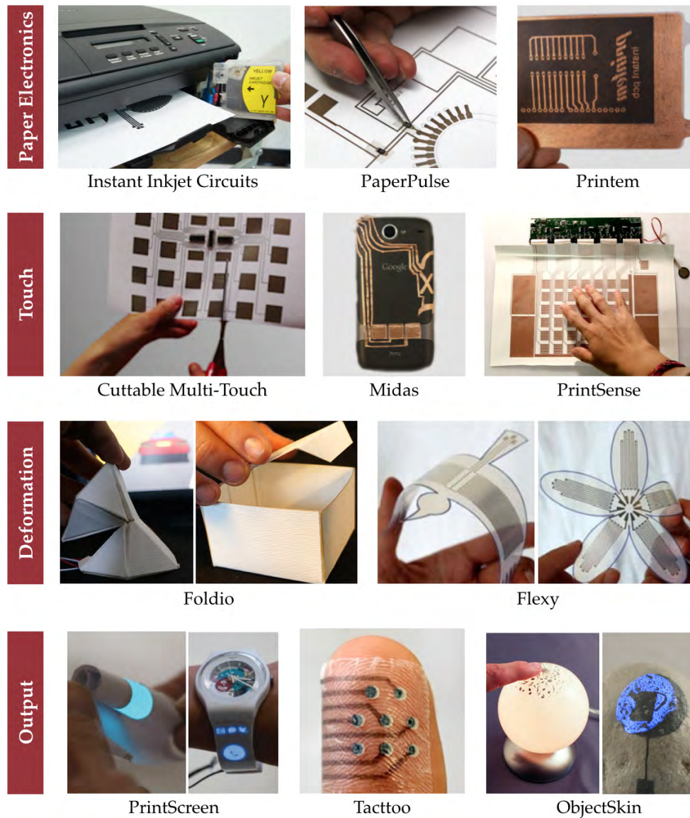
Figure 2.4: Examples of 2D-printed interactivity in the areas of paper electronics [Kaw+13; RTL15; CW15], touch [Olb+13; SZH12; Gon+14], deformation [Olb+15; VS17], and visual or haptic output [OWS14; WGS18; GS18].
