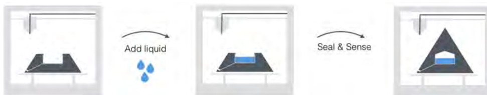
Figure 6.1: Fabrication process: (a) Start 3D printing, (b) stop & add liquid, (c) continue printing to seal object & sense tilting or motion.
