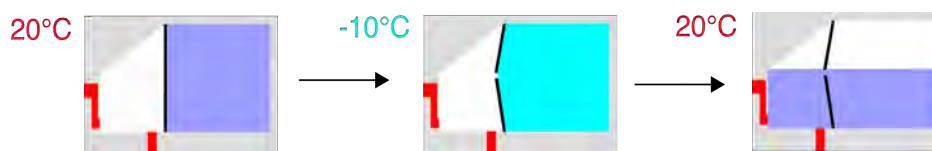
Figure 7.12: Due to the increased volume of a frozen liquid (middle), a thin wall breaks, resulting in the deposition of liquid into the left chamber.
