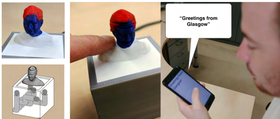
Figure 4.8: A 3D-printed prototype of a person, that is used to send a greeting notification to the corresponding person.
