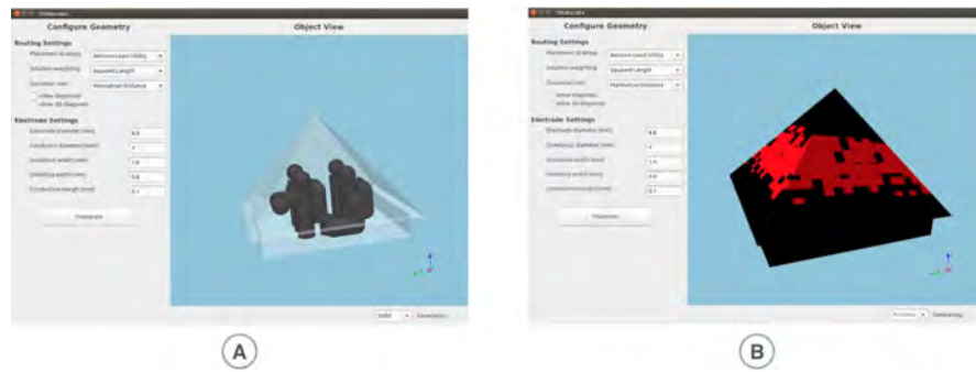
Figure 4.3: The TRILATERATE object generator: After loading a 3D model, trilateration sensors are generated (A). Users may inspect the expected accuracy (red equals high accuracy) using a heat map visualization (B).
