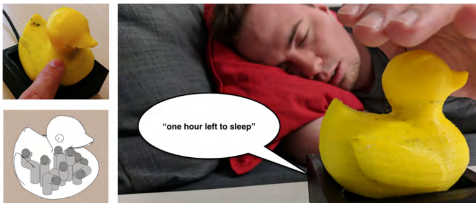
Figure 4.9: A prototype of a 3D-printed duck that acts as an alarm clock.
