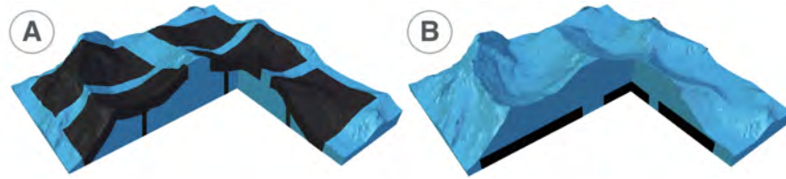
Figure 3.3: Cross-section of the Himalaya mountains model showing touch sensing with (a) curved electrodes on the surface, and (b) flat electrodes in the subsurface (black parts are touch-sensitive).
