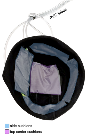
Figure 3: Actuator cushions in (a) deflated, and (b) inflated state.
