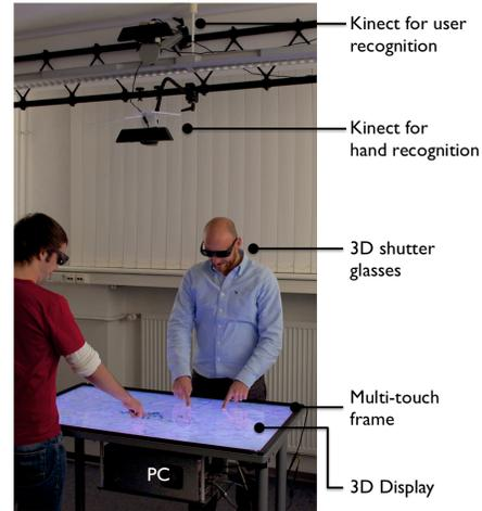
**Figure 2. Prototypical implementation of Permulin**
