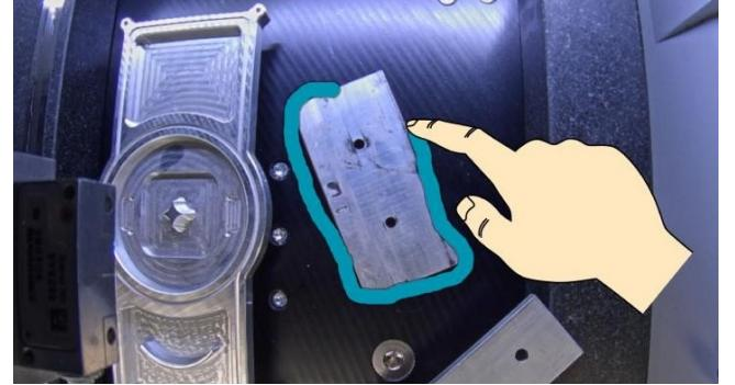
**Figure 5:** CaMea allows users to draw the outlines of a workpiece roughly onto the camera image. We use a template matching algorithm to extract the type of the shape.
