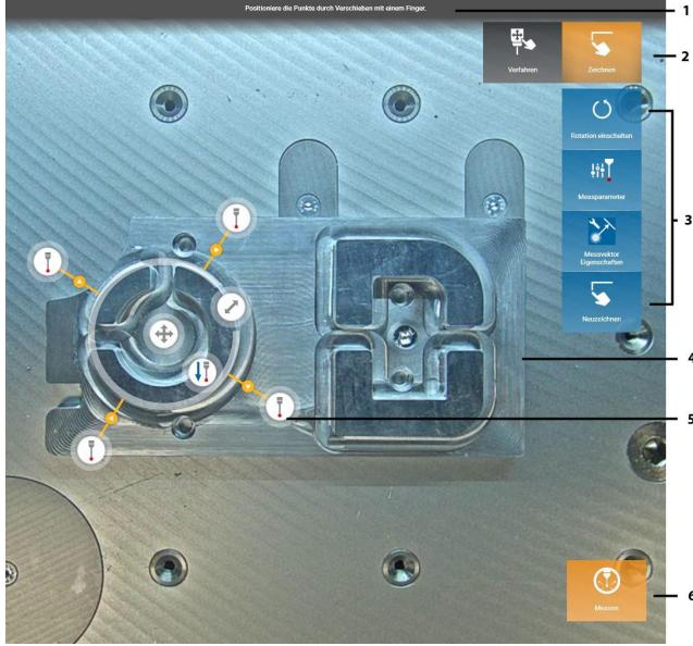
**Figure 4:** The user interface of CaMea superimposed on a workpiece. The user can intuitively select parts of the geometry and define probing points. The figure shows 1) Information text, 2) Mode Selection, 3) Option Buttons, 4) Workpiece, 5) Probing point handle and 6) Start measurement button.
