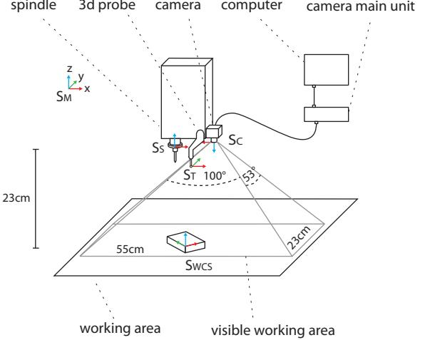
**Figure 3: We mounted the camera on the spindle inside the machine. The machine coordinate system  $S_M$  is the frame of reference. The camera coordinate system  $S_C$  relative to  $S_S$  is calculated in the camera calibration. The workpiece coordinate system  $S_{WCS}$  relative to  $S_M$  is measured in the workpiece measurement step.**
