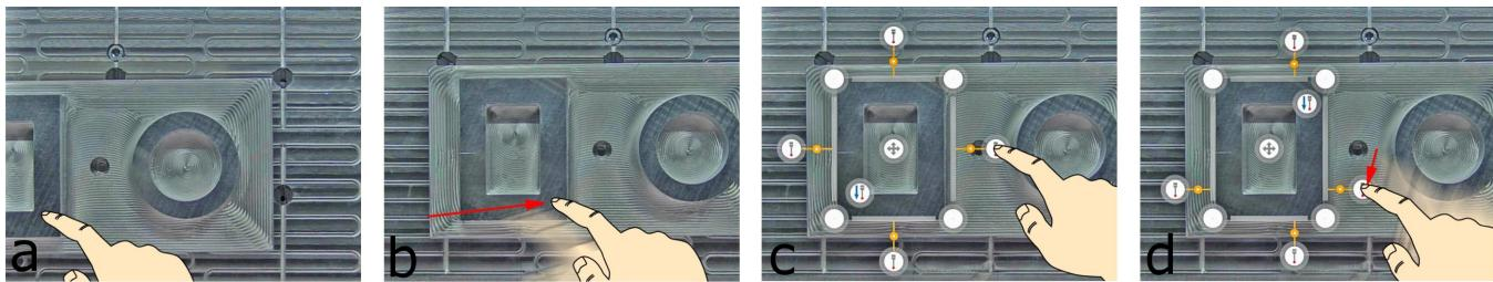
Figure 1: CaMea supports users in the process of initializing a workpiece in a CNC milling machine. We mounted a camera inside the machine and allow the user to move (a,b) the camera though touch gestures to align the camera with the workpiece. Once aligned, the user can select (c) and move (d) the touch points for the probing tip on screen.
