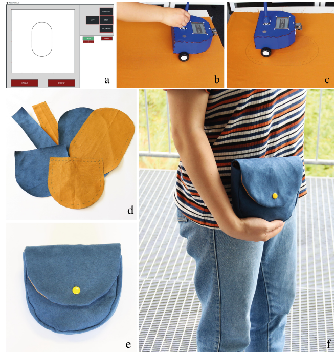
Figure 14: Creating sewing patterns on fabric: a) uploading the design, b) scaling the design on the fabric, c) the robot prints the pattern on the fabric, d) cutouts with sewing marks, e and f) fabricated clutch bag.
