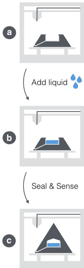
**Figure 1:** Fabrication process: (a) Start 3D printing, (b) stop & add liquid, (c) continue printing to seal object & sense tilting or motion.
