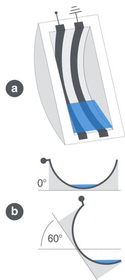
**Figure 2:** (a) 3D and (b) 2D view of halfpipe pattern filled with liquid.
