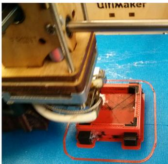
**Figure 4:** 3D printing of cubic pattern with liquid already filled in.
