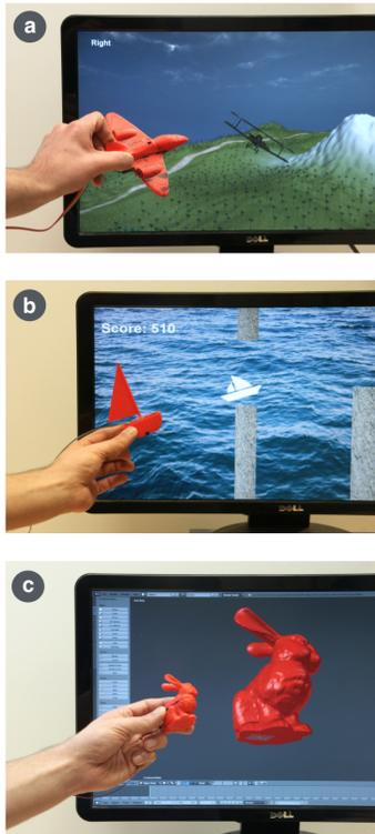
**Figure 6:** Interactive example applications: (a) flying an airplane simulation, (b) avoiding obstacles with a physical ship, and (c) rotating a physical object for 3D navigation.
