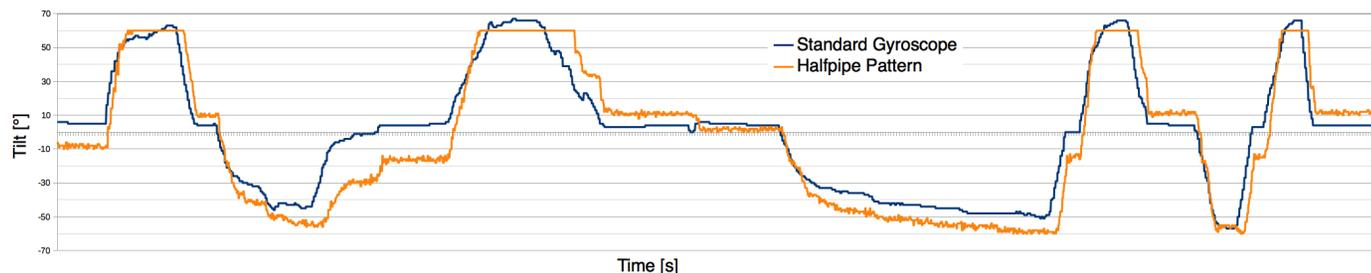
**Figure 8:** Comparison between tilts reported by the halfpipe pattern (orange) versus a MPU 6050 tilt sensor (blue) over a timeframe of 184s.
