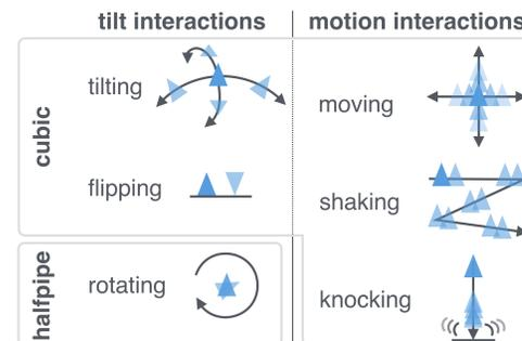
**Figure 5:** Illustration of various tilt and motion interactions supported by the cubic or halfpipe pattern.
