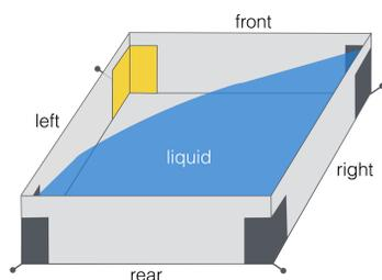
**Figure 3:** Tilted cubic pattern. One of the four electrodes is triggered due to lack of liquid.
