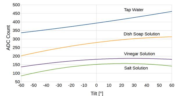
**Figure 7:** Trend lines for tap water, dish soap solution, vinegar solution, and salt solution showing the dependency between ground-truth tilt and measured counts for the halfpipe pattern.
