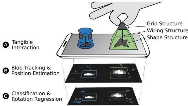
**Figure 2: Based on the user’s interaction (A), Itsy-Bits identifies and tracks blobs in the capacitive image (B) and classifies the conductive shape, its size, and its orientation using machine learning (C).**
