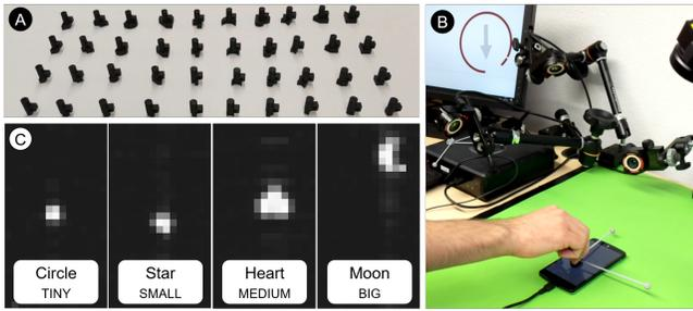
**Figure 6:** For the data collection study, we printed test objects of all conductive shapes and sizes (A) and recorded their position and rotation on the touchscreen with optical tracking (B) together with the corresponding capacitive images (C).
