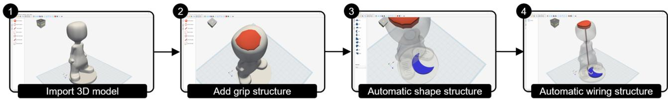
**Figure 4: Using a design tool, non-expert users (1) import a 3D-printable model and add (1) grip and (2) shape structures. The tool then automatically embeds necessary wires (4) and provides an export of 3D models for multi-material printing.**
