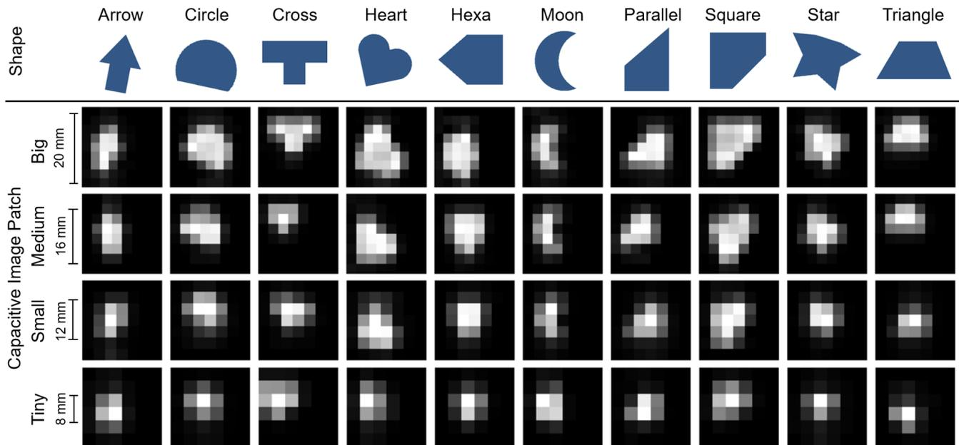
**Figure 5: The set of 10 rotation-variant shapes (named after the shape it originated from) and a sample of a corresponding BIG (20 × 20 mm), MEDIUM (16 × 16 mm), SMALL (12 × 12 mm), and TINY (8 × 8 mm) capacitive image.**
