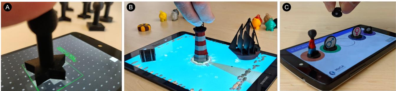
**Figure 1:** Itsty-Bits recognizes 3D-printed tangibles as small as a fingertip via the capacitive image of an embedded conductive shape (A). This opens up a variety of tangible user interfaces on the most common form factors of touchscreens, such as individualized interactive board games (B) or a more tangible learning experience (C).
